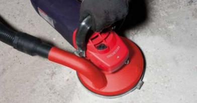
The **SPARKY** range of grinders offers three different body types, short, medium and long bodied, covering from 750 to 2600W and disc sizes 115mm-125mm-150mm-180mm-230mm. All grinders have a light and robust magnesium alloy gearbox and milled, case hardened gears from our own production.
