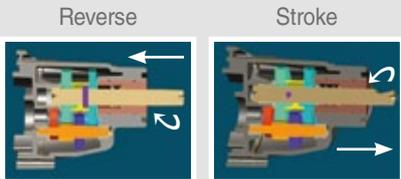
Mechanical mechanism for reversing the machine after threading
